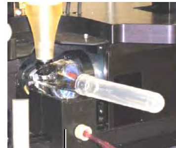
Debubble reservoir located on the flush bucket during a wet shutdown
