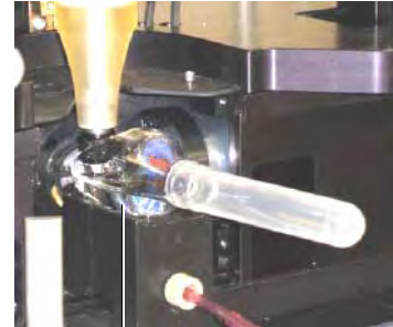
Debubble reservoir with DI water used to submerge a nozzle tip during a wet shutdown
